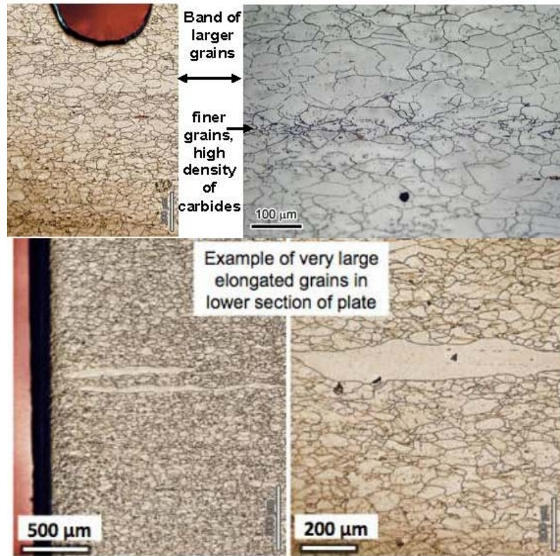
Figure 4.2. Optical micrographs illustrating microstructural variations due to compositional banding in an Alloy 690 plate material [14].
