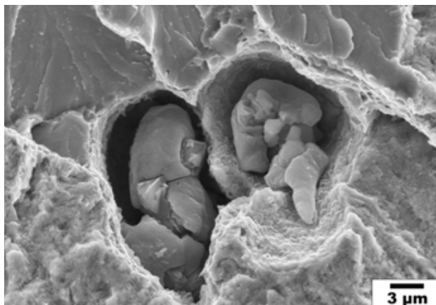
Figure 5.12. Partially dissolved MnS inclusions on the crack surface [100].
