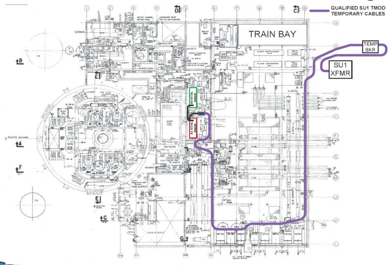
> Temporary breaker supplying power to vital switchgear from SU1 transformer
