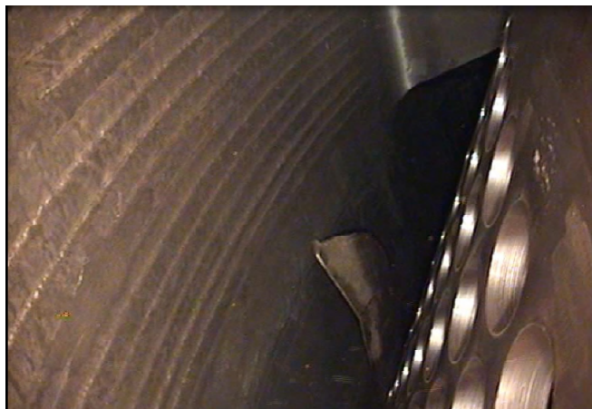
View of the impeller piece looking down from above the flow skirt
