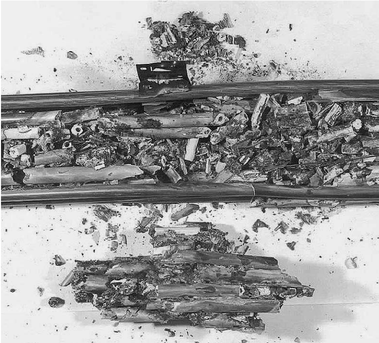
Figure 1. Section of the Test Bundle from PWR FLECHT Run 9573 that Incurred Runaway Oxidation
