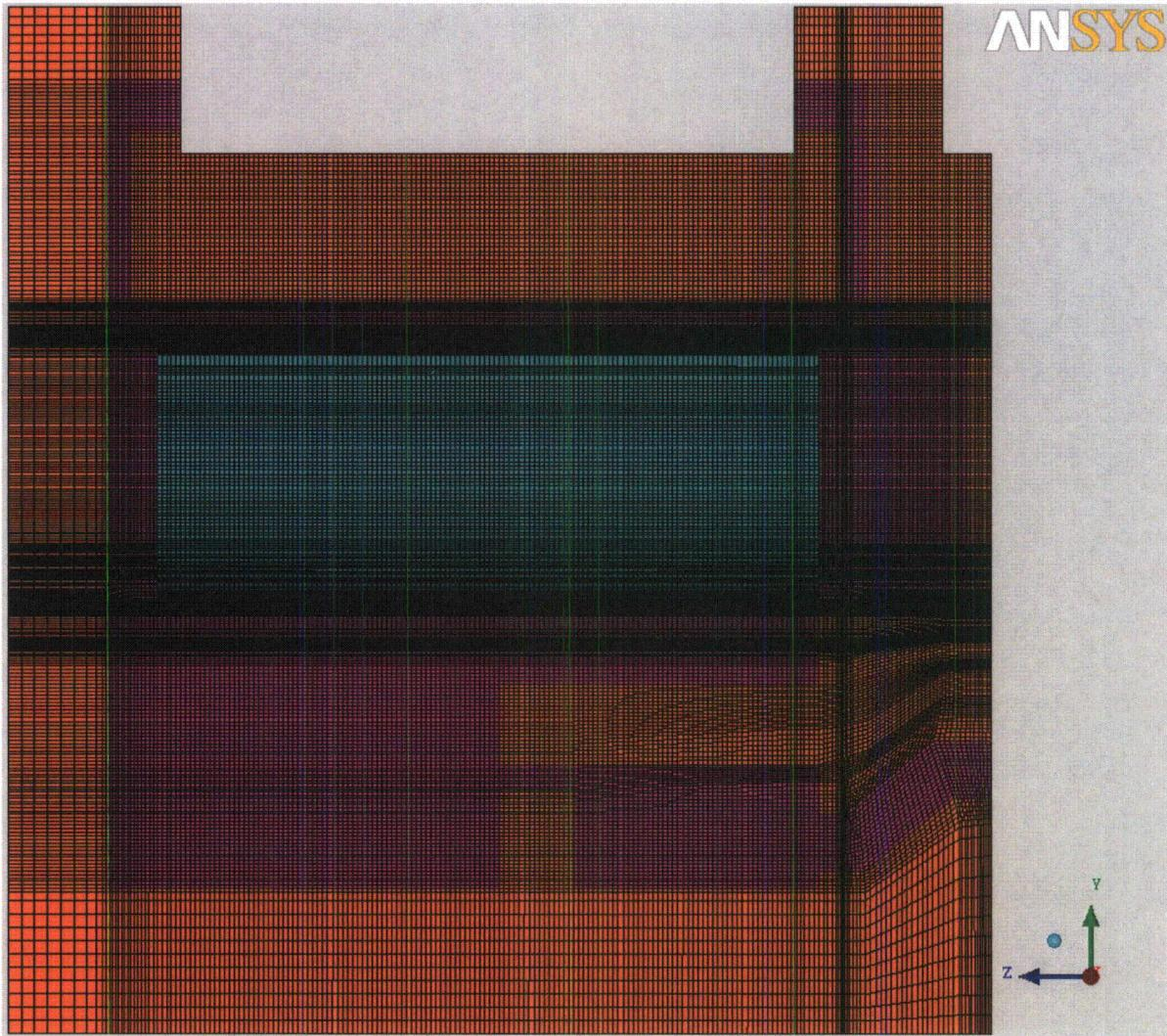
**Figure 5-2: Axial View of the Hexahedral Mesh on the Symmetrical Mid-plane for CCNPP HSM and DSC.**
