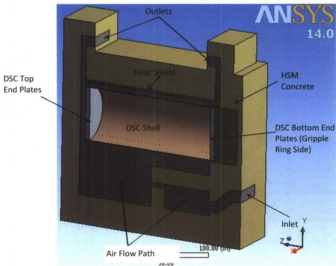
**Figure 5-1: CCNPP HSM with 24P/32P DSC Shell and End Plates**
