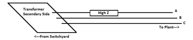
A high impedance in series with one phase on the 4.16kV system will be detected because of running motor loads on the buses. The high impedance would be similar to a single open
