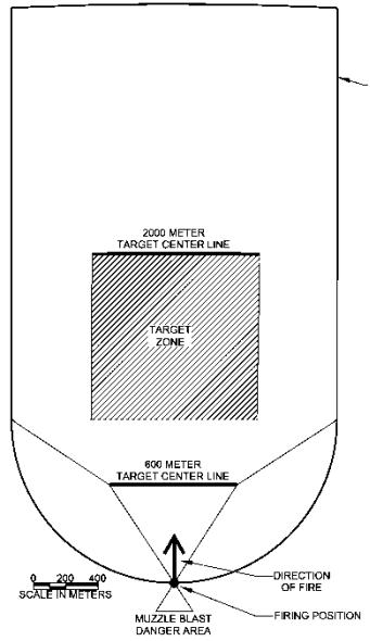
Figure 1: Radiation Control Area Based on Firing Characteristics
