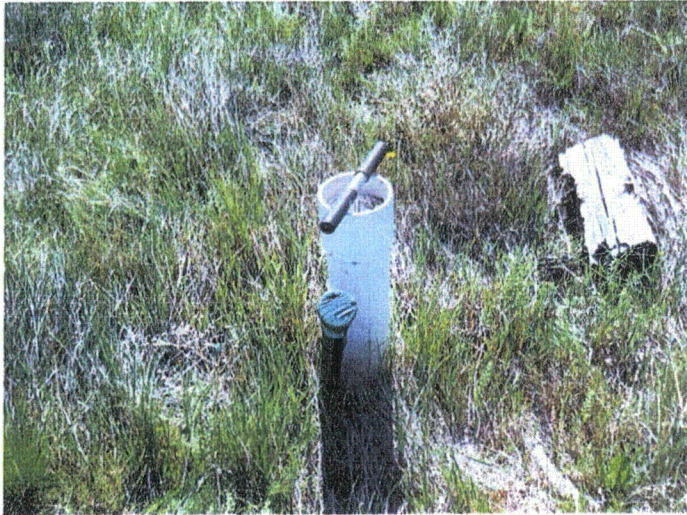
Figure 17b, Uncapped well in MU-H
