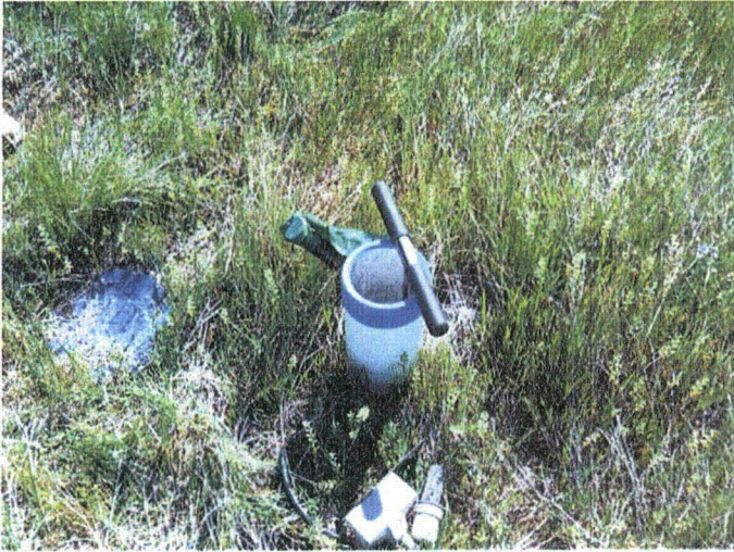
Figure 17a Uncapped well in MU-H
