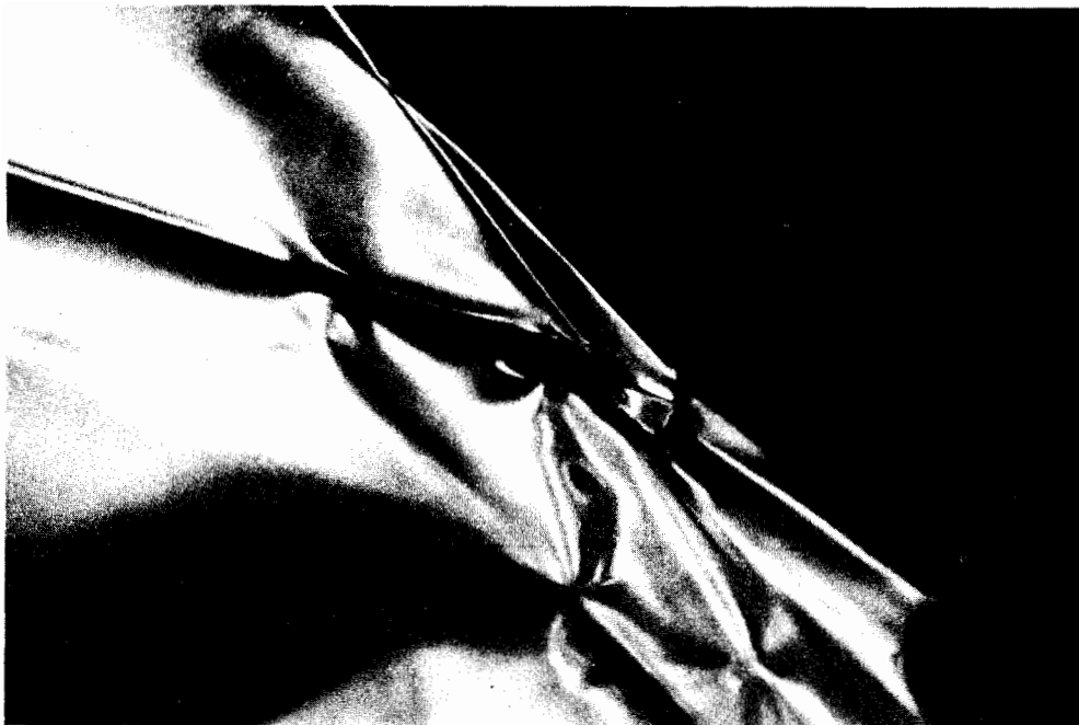
FRACTURE CAUSED BY WATER PRESSURE
