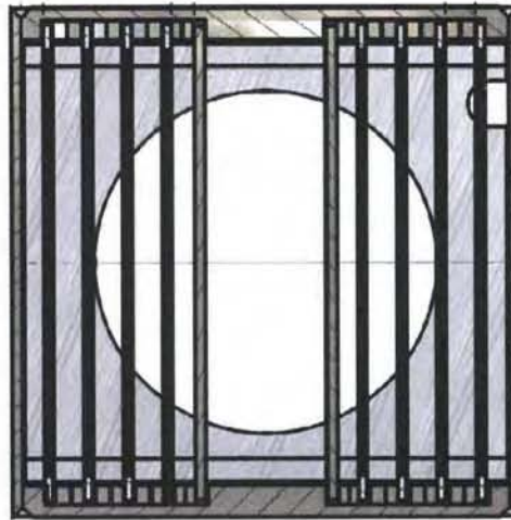
Figure 4-28: Control LEU fuel assembly.
