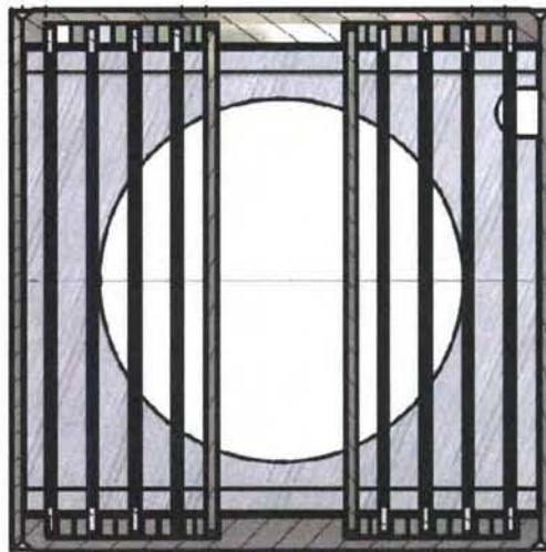
Figure 4-6: Control fuel assembly.
