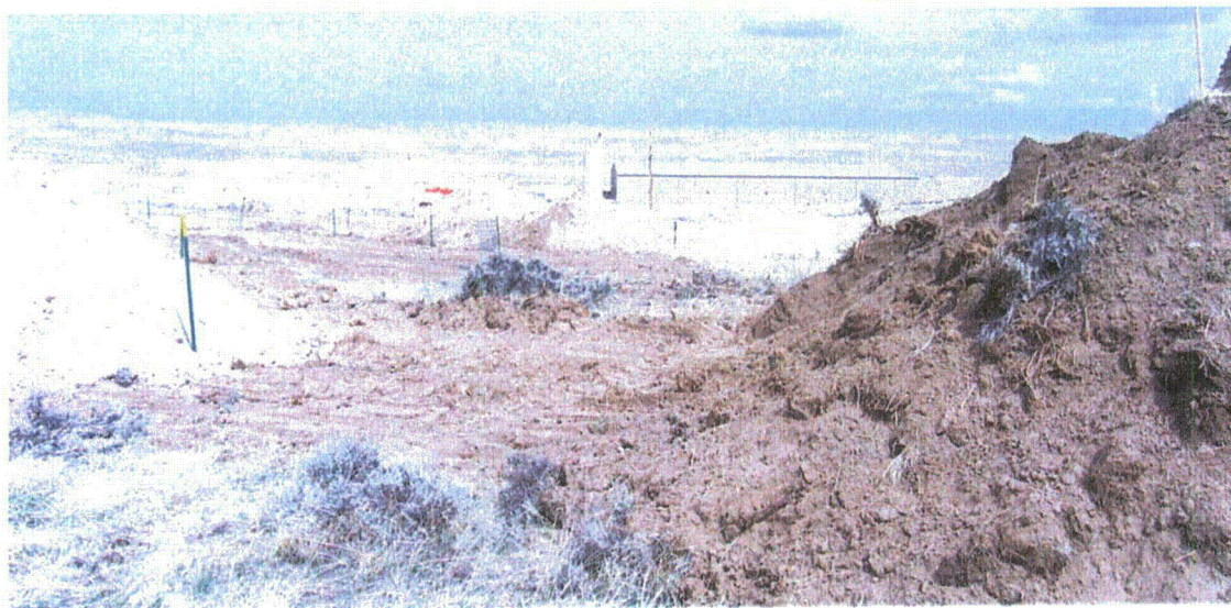
Figure 8 Topsoil pile in MU-10 without erosion control or protection from mine disturbances
