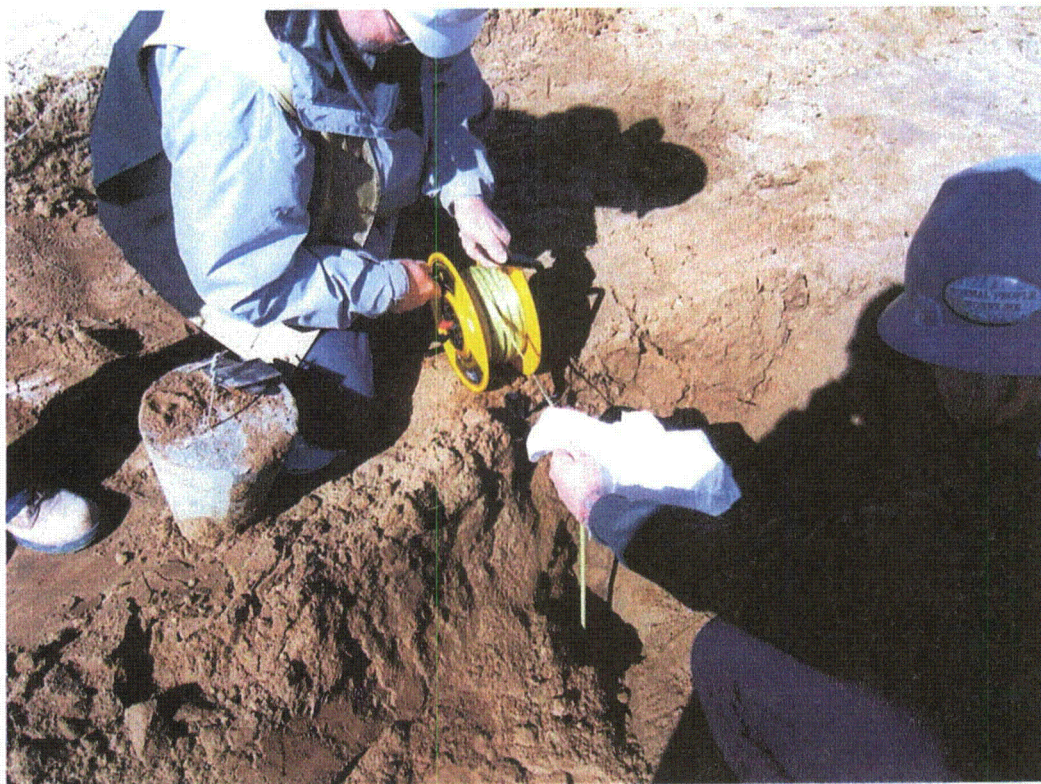
Figure 2 – Measuring depth to plug gel
