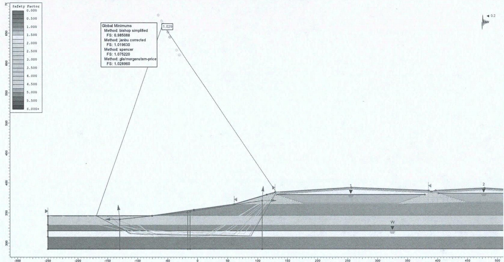
**Figure E5.** Determination of yield acceleration assuming the lower sand layer in fully-liquefied state (wedge failure surface).
