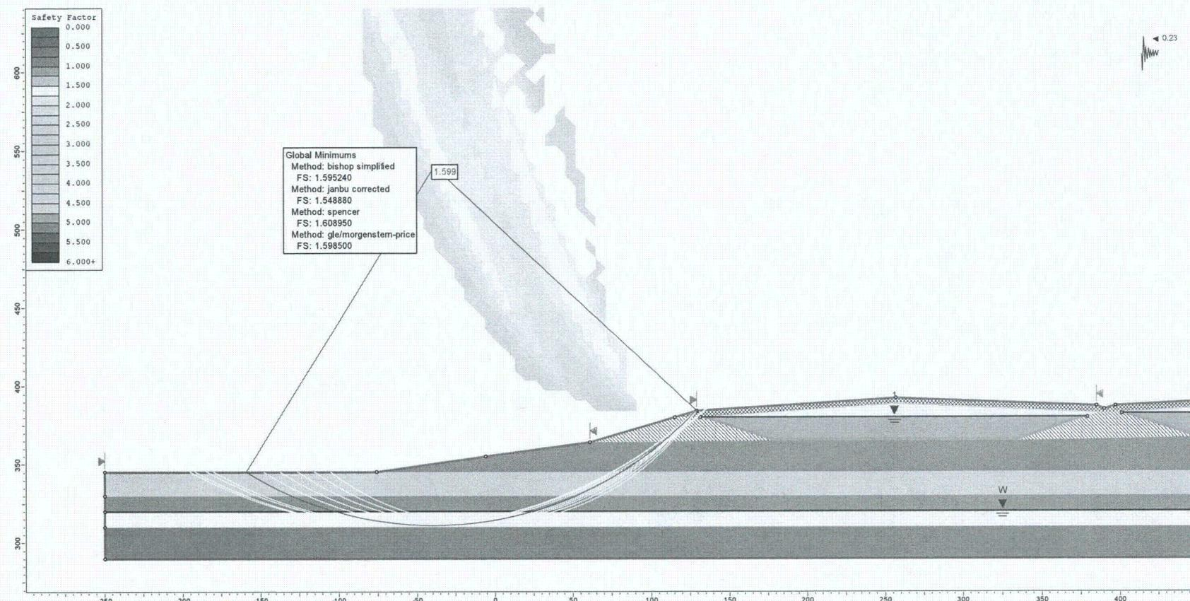
**Figure F3.** Pseudo static analysis of the exterior berm in a 475-year event assuming partly liquefied state in the lower sand (circular failure surface,  $k_h = 0.67 \times \text{PGA}$ ).
