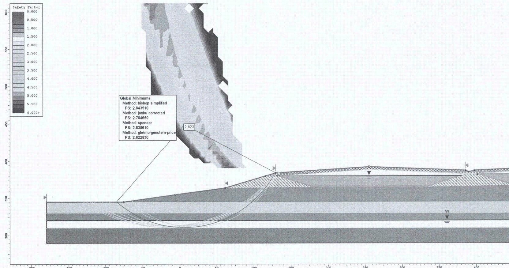
**Figure E2.** Post-liquefaction stability of the exterior berm assuming the lower sand layer in fully-liquefied state (circular failure surface).
