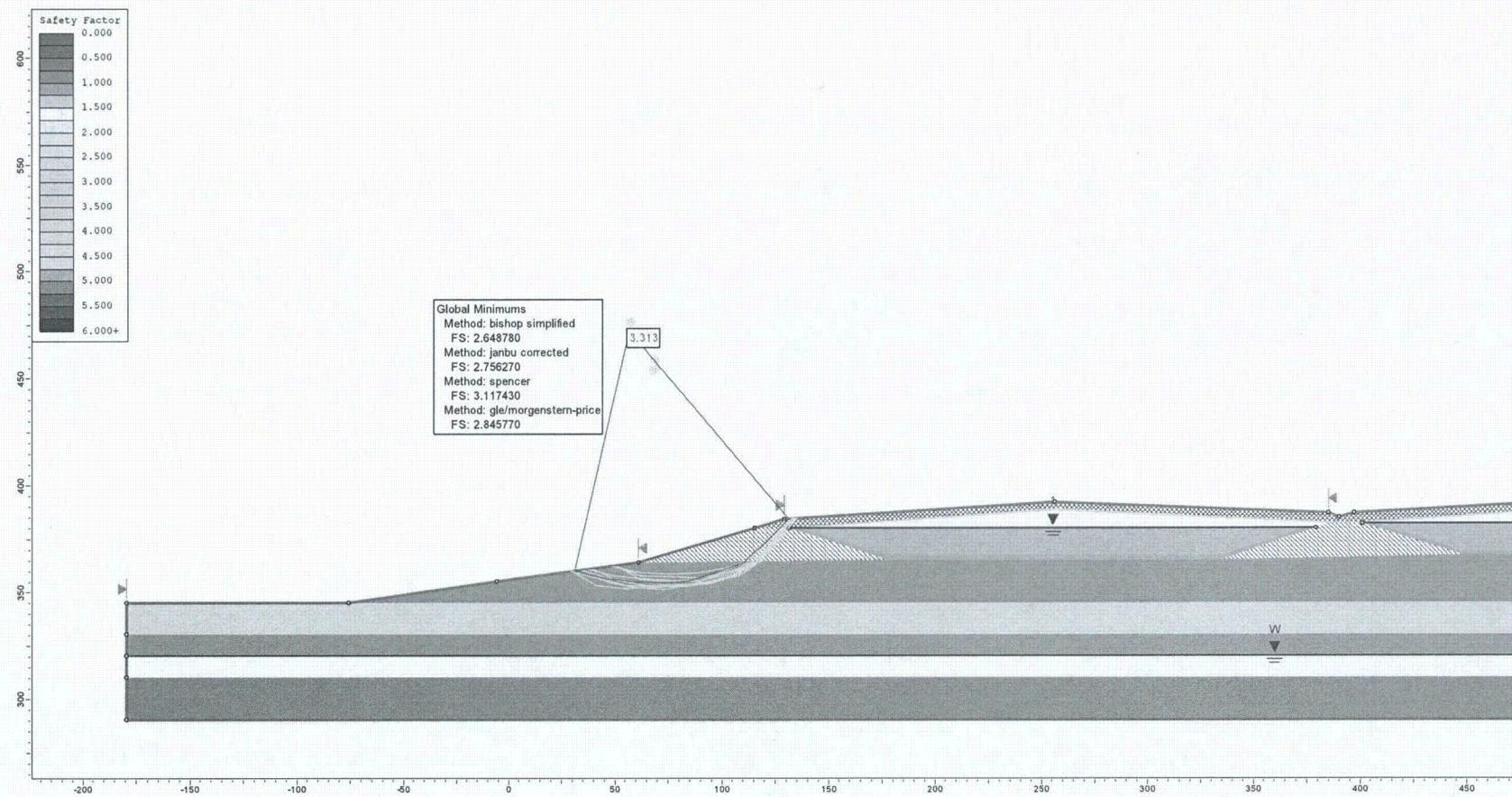
**Figure E1.** Post-liquefaction stability of the exterior berm assuming the lower sand layer in fully-liquefied state (non-circular failure surface).
