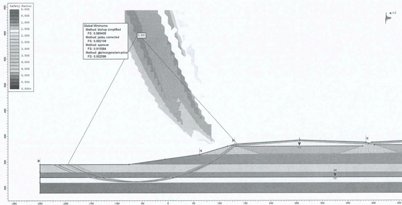
**Figure F21.** Pseudo static analysis of the exterior berm in a 2475-year event assuming partly liquefied state in the lower sand (circular failure surface,  $k_h = 0.5 \times \text{PGA}$ ).
