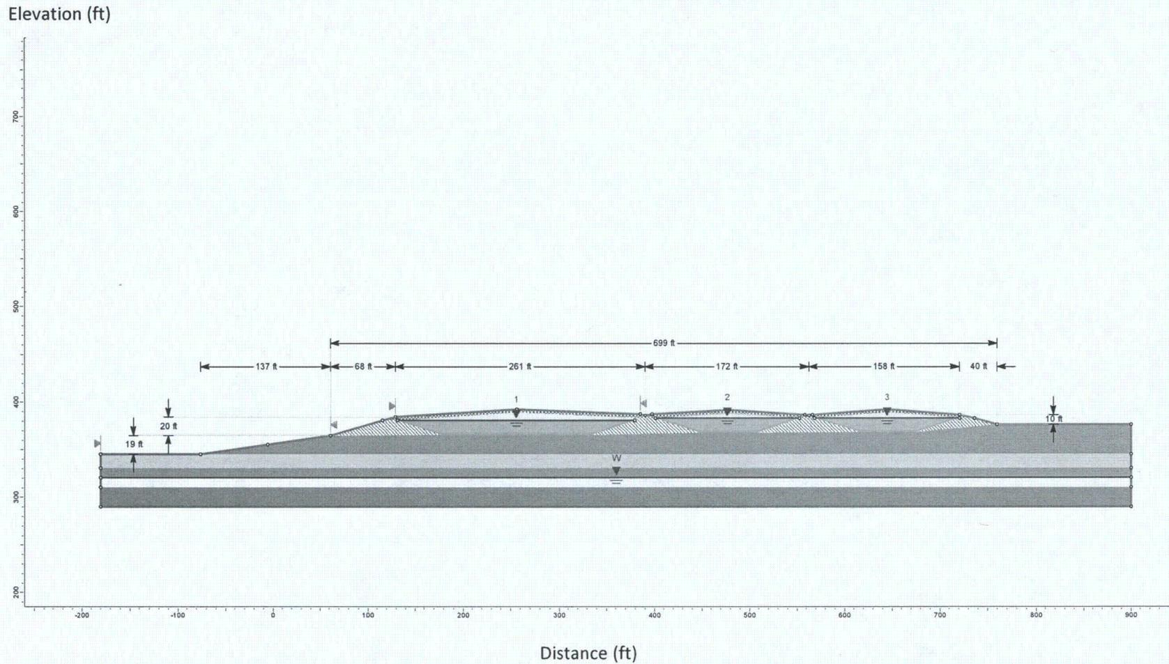
**Figure D1.** Cross section A-A showing subsurface and groundwater conditions.
