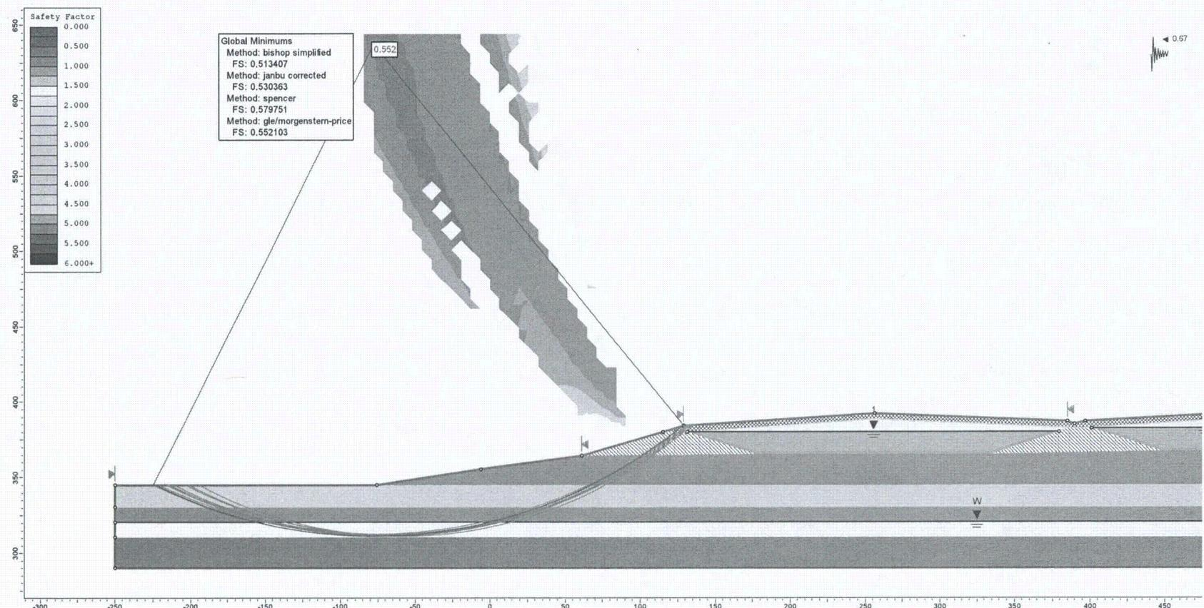
**Figure F13.** Pseudo static analysis of the exterior berm in a 2475-year event assuming full liquefaction in the lower sand (circular failure surface,  $k_h = 0.67 * \text{PGA}$ ).
