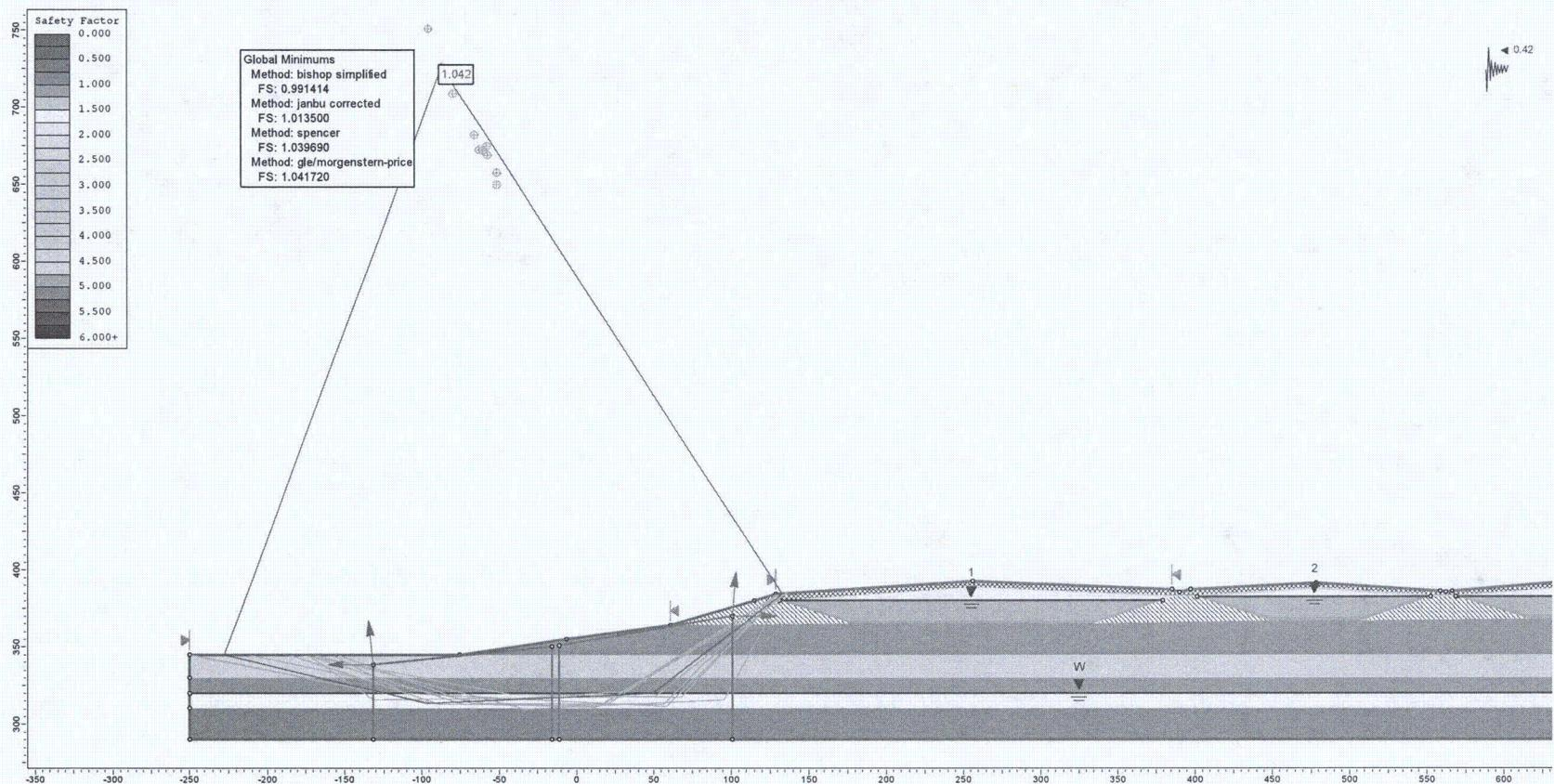
**Figure E11.** Determination of yield acceleration assuming the lower sand layer in fully-liquefied state (wedge failure surface).
