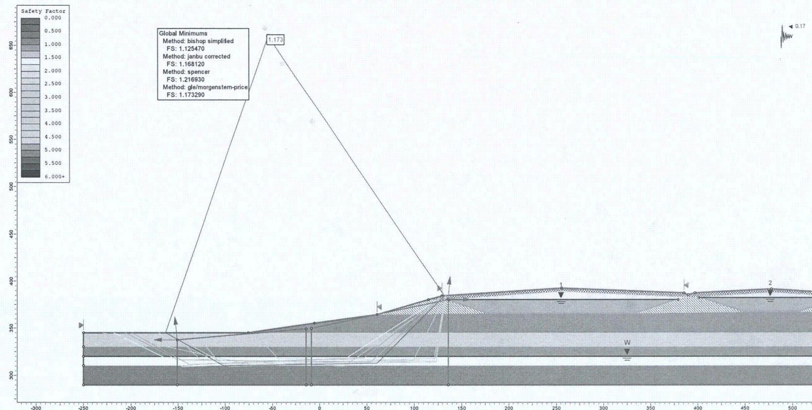
**Figure F8.** Pseudo static analysis of the exterior berm in a 475-year event assuming full liquefaction in the lower sand (wedge failure surface,  $k_h = 0.5 * \text{PGA}$ ).
