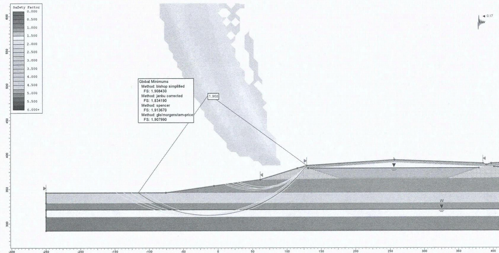
**Figure F9.** Pseudo static analysis of the exterior berm in a 475-year event assuming partly liquefied state in the lower sand (circular failure surface,  $k_h = 0.5 * \text{PGA}$ ).
