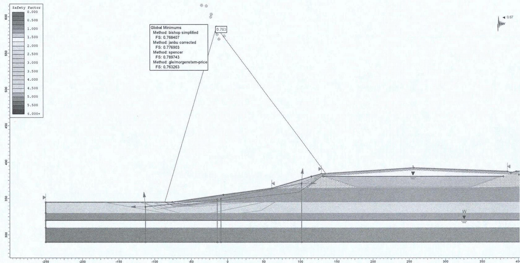
**Figure F18.** Pseudo static analysis of the exterior berm in a 2475-year event assuming no liquefaction in the lower sand (wedge failure surface,  $k_h = 0.67 * \text{PGA}$ ).
