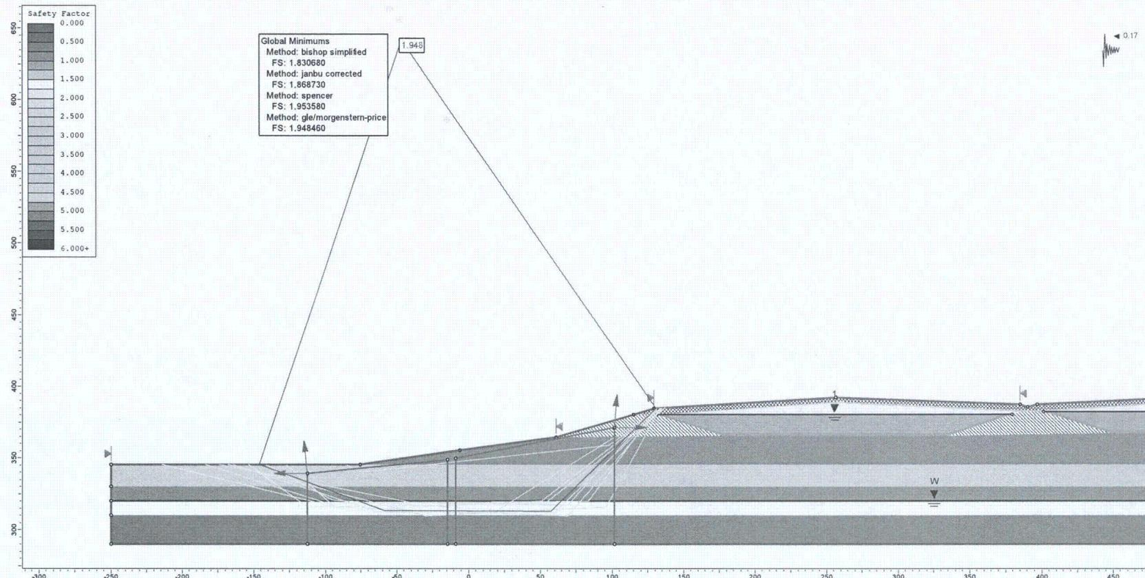
**Figure F10.** Pseudo static analysis of the exterior berm in a 475-year event assuming partly liquefied state in the lower sand (wedge failure surface,  $k_h = 0.5 * \text{PGA}$ ).
