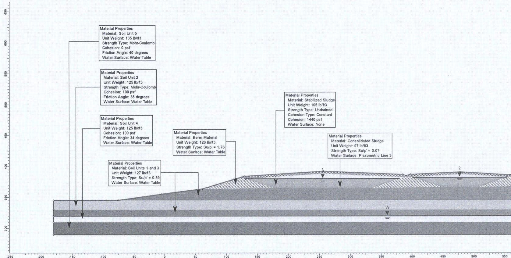
**Figure D3.** Soil properties for seismic stability analysis assuming no liquefaction in the lower sand layer (Soil Unit 4).
