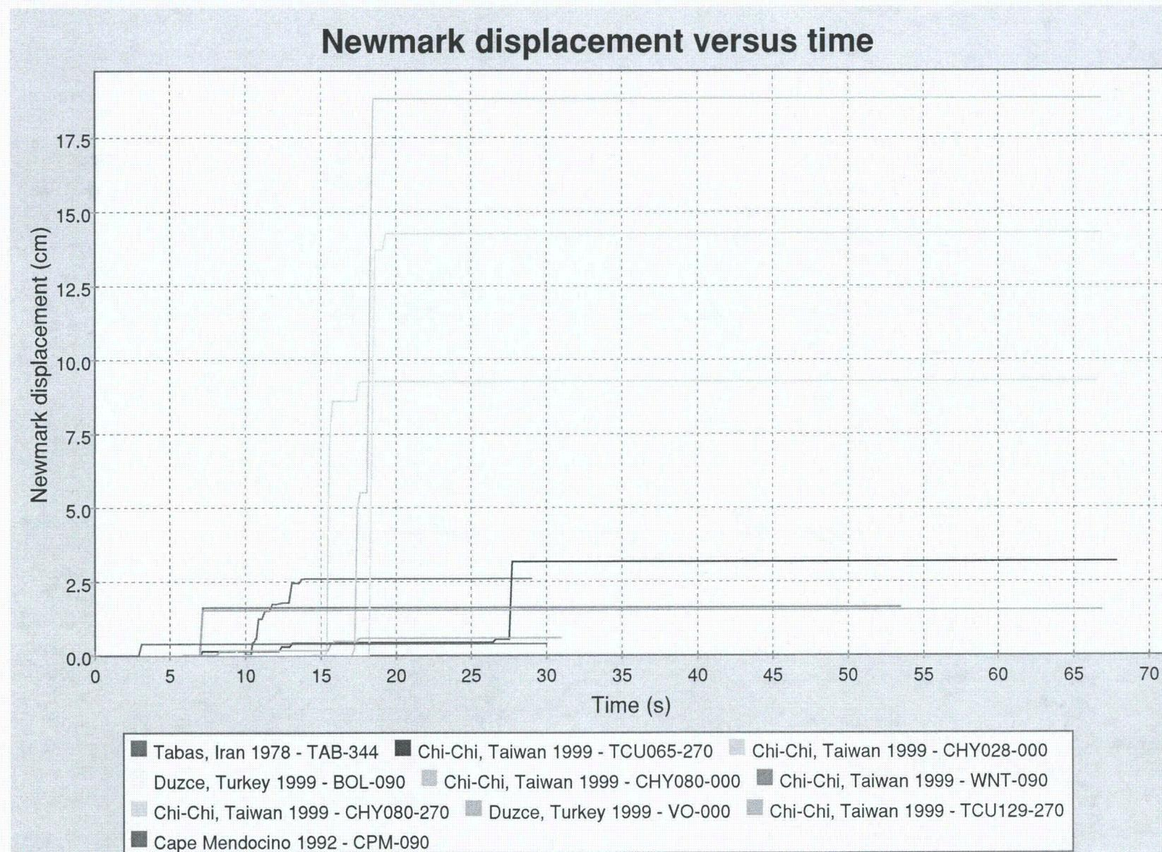
Figure E20. Permanent Deformation Based on Bray and Travasarou (2007)
