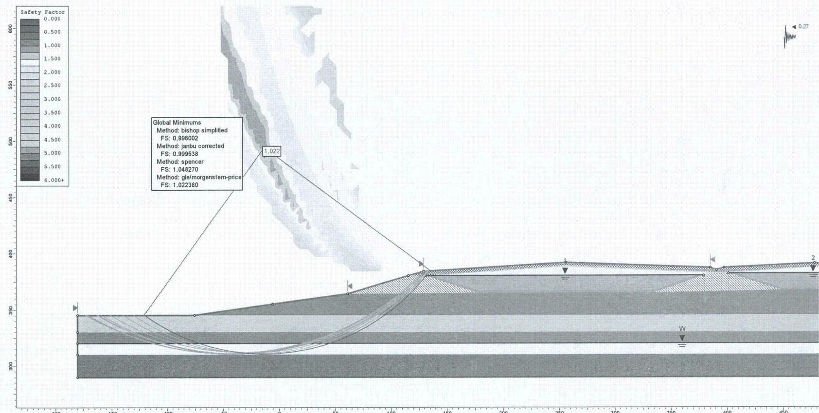
**Figure E4.** Determination of yield acceleration assuming the lower sand layer in fully-liquefied state (circular failure surface).
