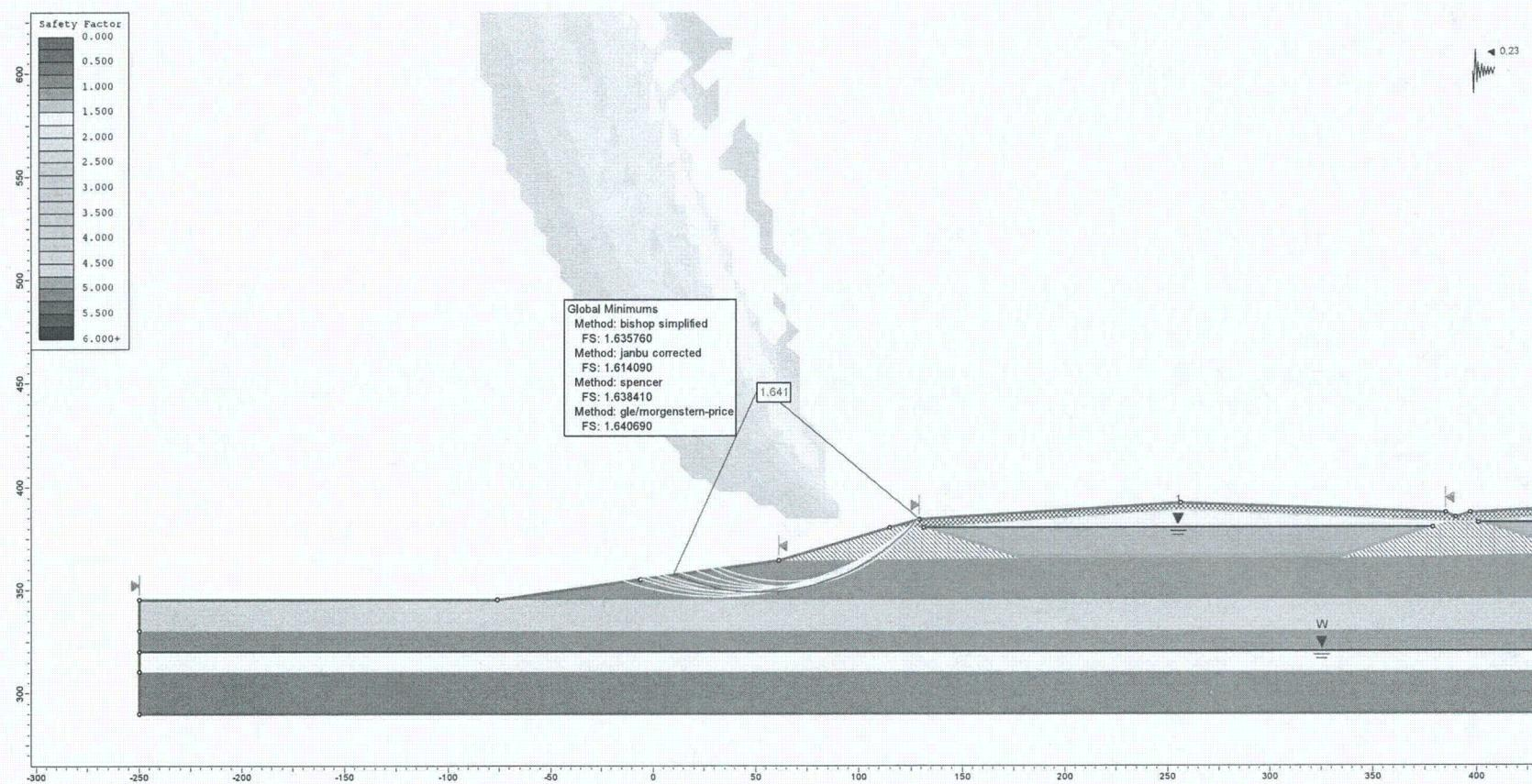
**Figure F5.** Pseudo static analysis of the exterior berm in a 475-year event assuming no liquefaction in the lower sand (circular failure surface,  $k_h = 0.67 * \text{PGA}$ ).
