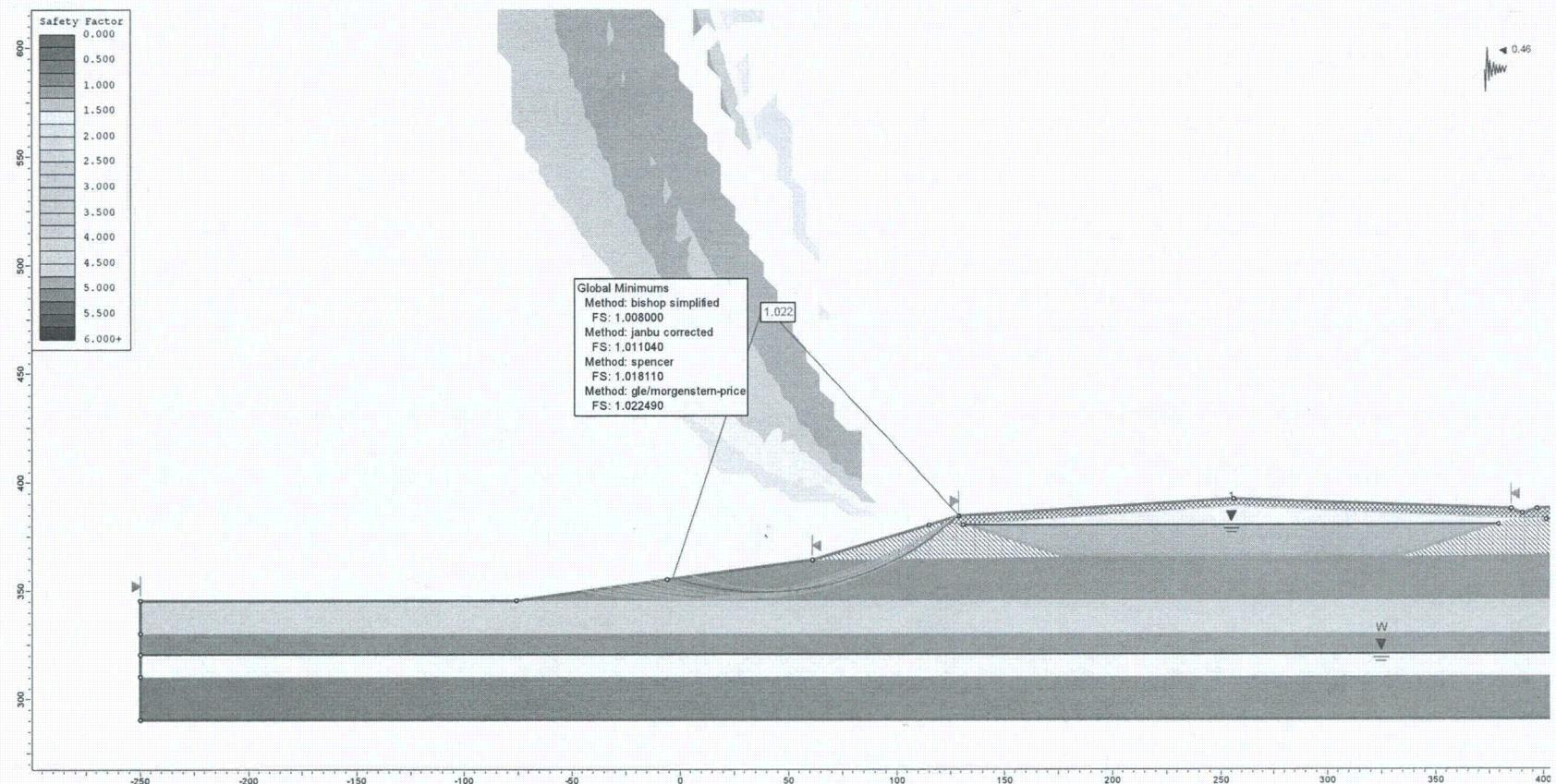
**Figure E16.** Determination of yield acceleration assuming the lower sand layer in non-liquefied state (circular failure surface).
