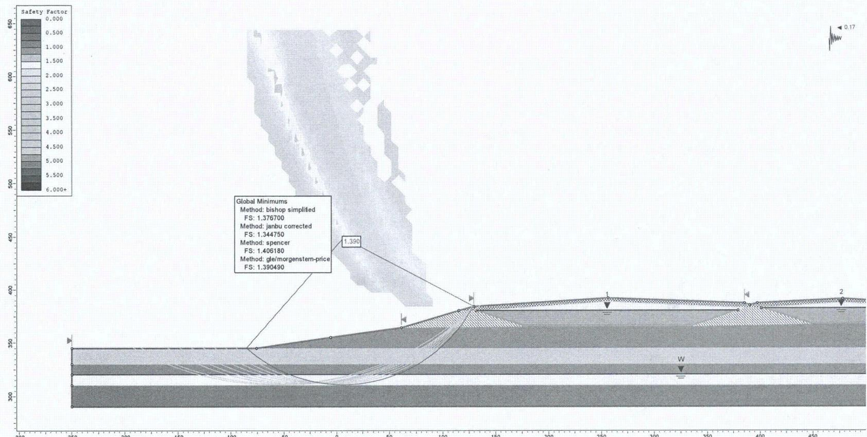
**Figure F7.** Pseudo static analysis of the exterior berm in a 475-year event assuming full liquefaction in the lower sand (circular failure surface,  $k_h = 0.5 * \text{PGA}$ ).
