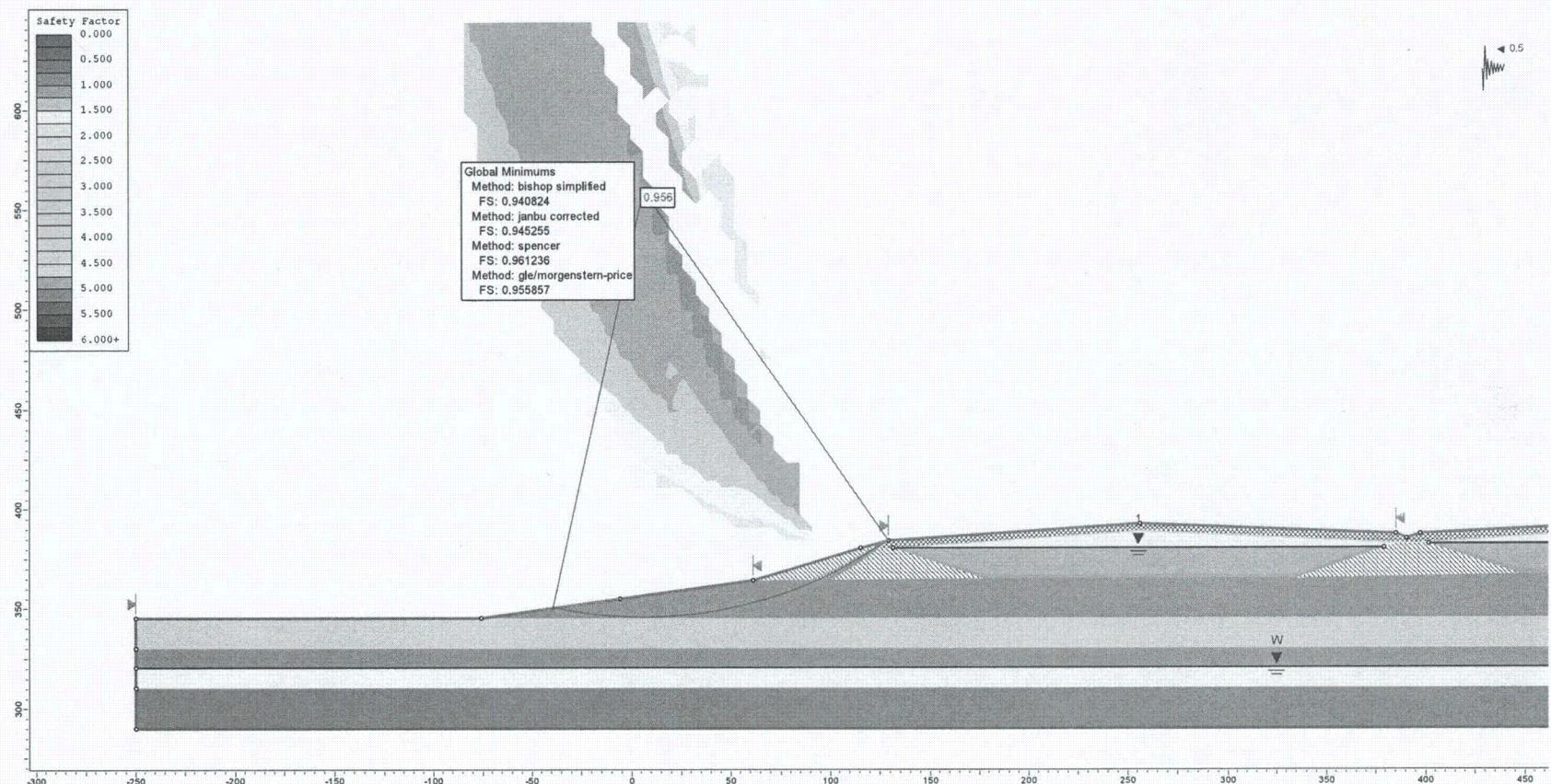
**Figure F23.** Pseudo static analysis of the exterior berm in a 2475-year event assuming no liquefaction in the lower sand (circular failure surface,  $k_h = 0.5 * \text{PGA}$ ).
