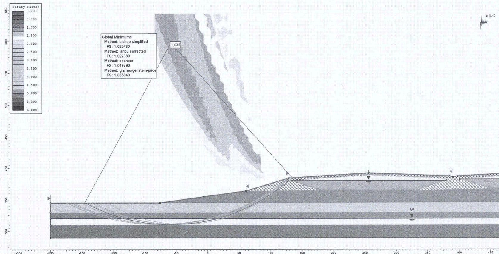
**Figure E10.** Determination of yield acceleration assuming the lower sand layer in fully-liquefied state (circular failure surface).
