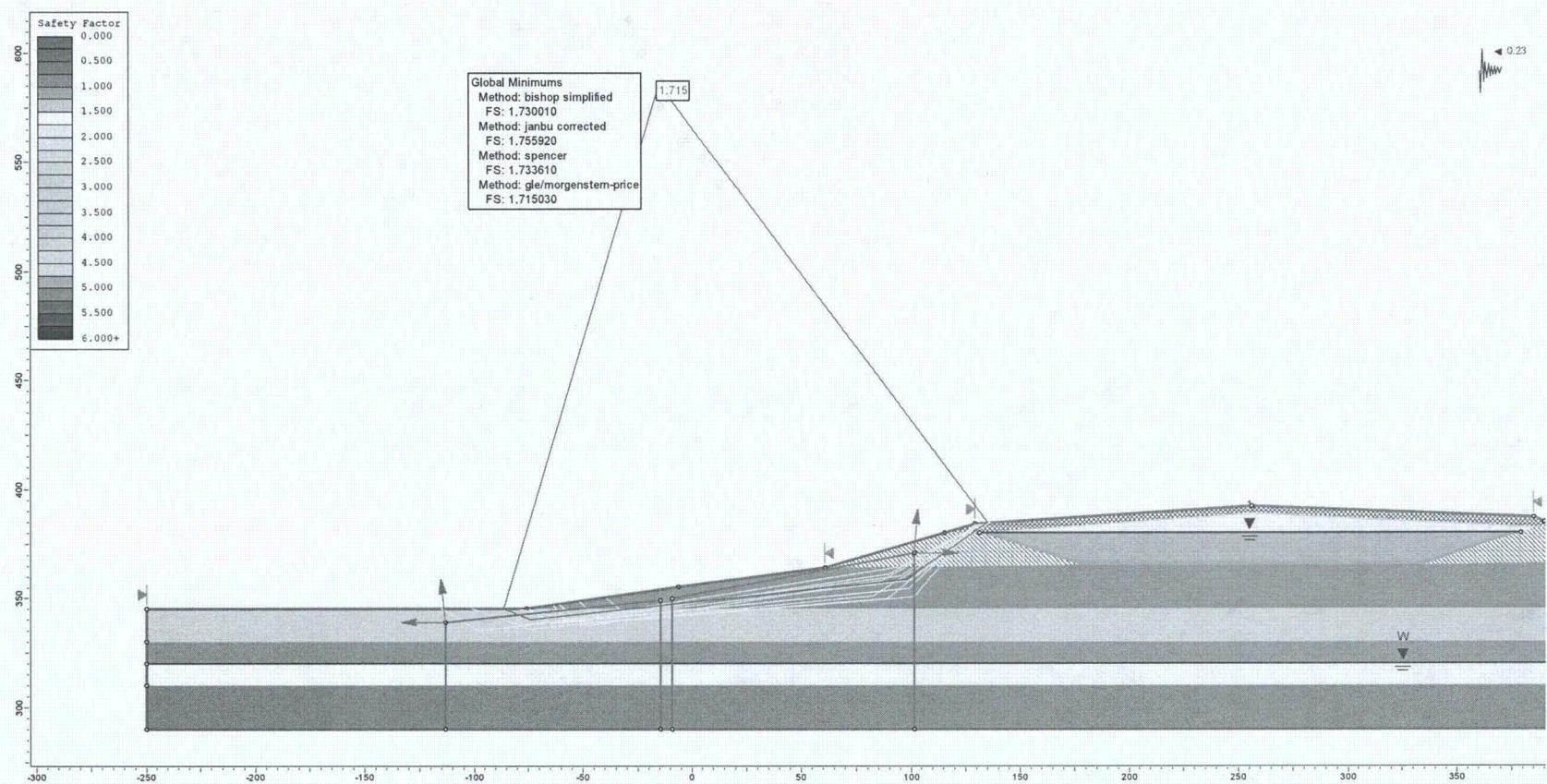
**Figure F6.** Pseudo static analysis of the exterior berm in a 475-year event assuming no liquefaction in the lower sand (wedge failure surface,  $k_h = 0.67 * \text{PGA}$ ).
