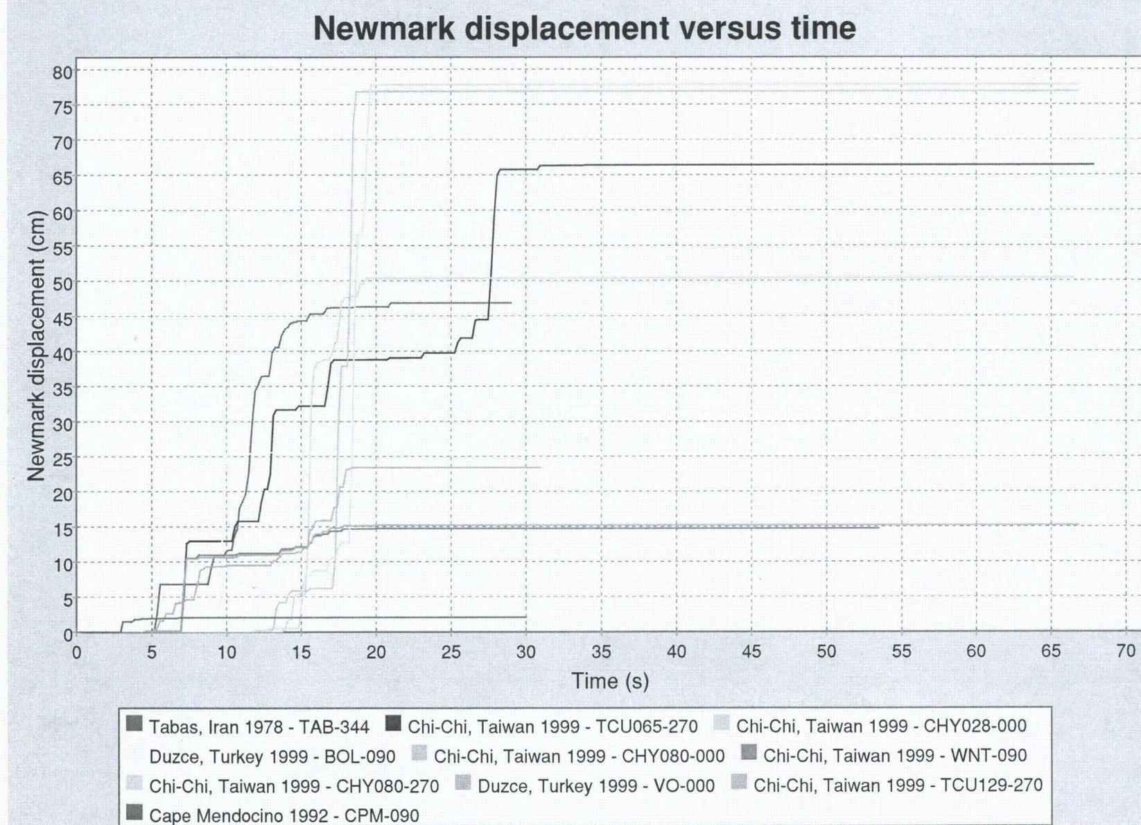
Figure E8. Permanent Deformation Based on Bray and Travasarou (2007)
