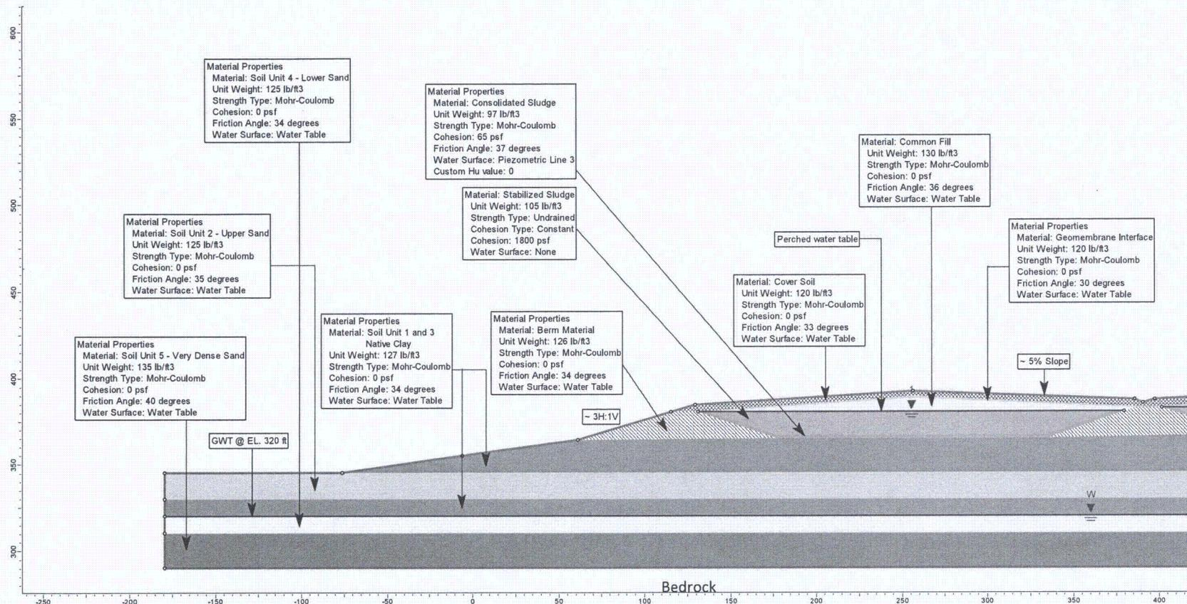
Figure D2. Static soil properties used in (long-term) condition.
