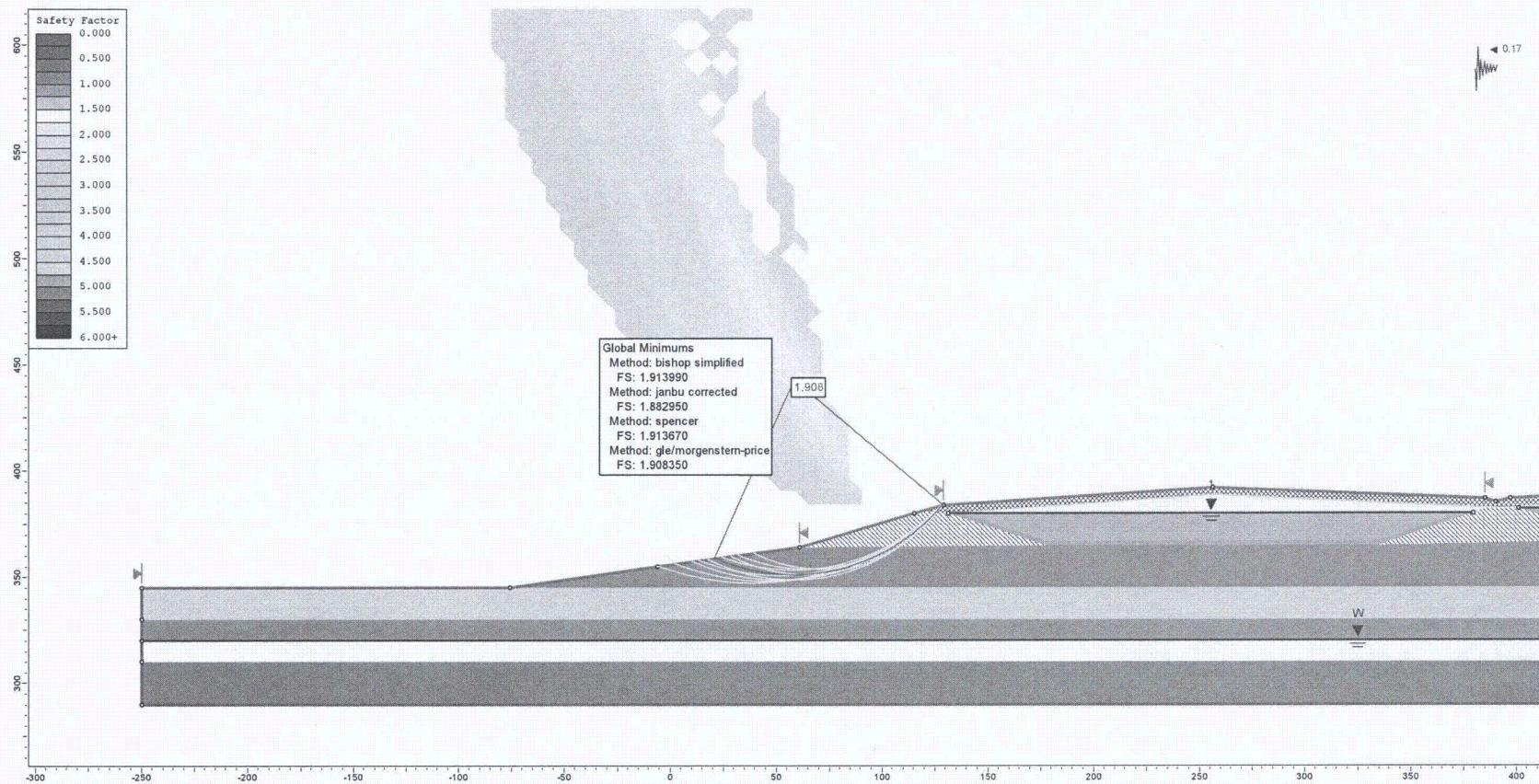
**Figure F11.** Pseudo static analysis of the exterior berm in a 475-year event assuming no liquefaction in the lower sand (circular failure surface,  $k_h = 0.5 * \text{PGA}$ ).
