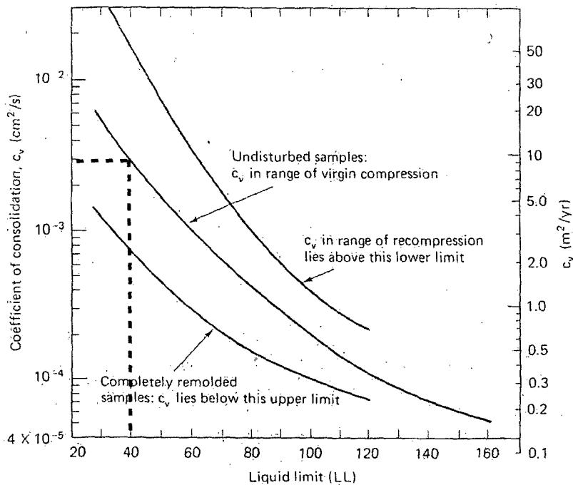
Fig. 9.10 Approximate correlations of the coefficient of consolidation  $c_v$  with the liquid limit (after U.S. Navy, 1971).
