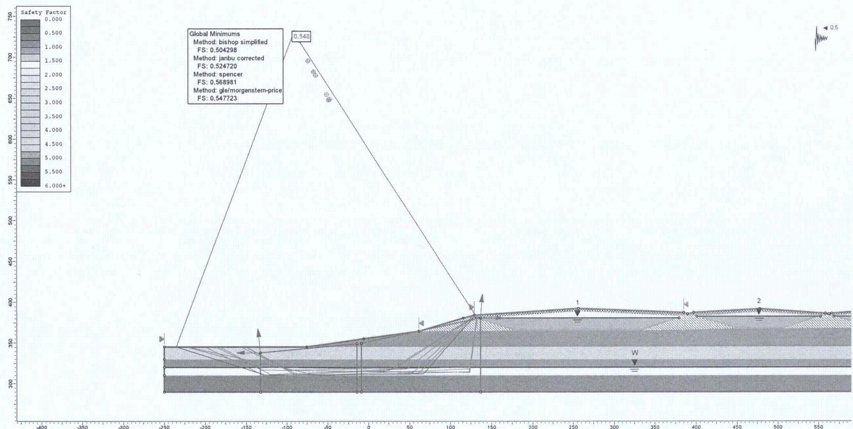
**Figure F20.** Pseudo static analysis of the exterior berm in a 2475-year event assuming full liquefaction in the lower sand (wedge failure surface,  $k_h = 0.5 \times \text{PGA}$ ).
