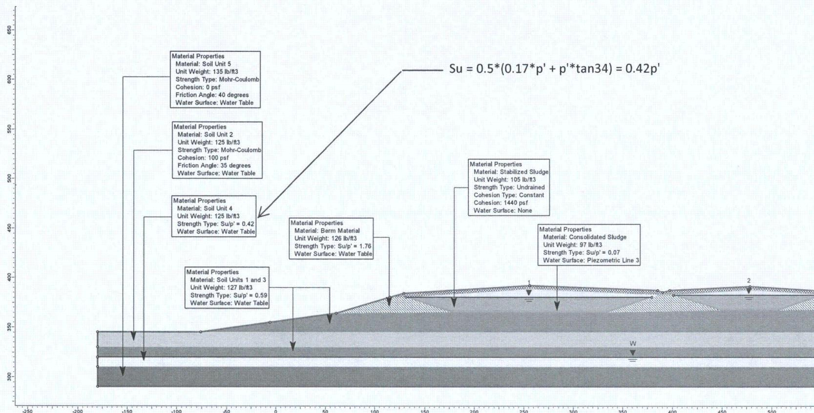
**Figure D5.** Soil properties for seismic stability analysis assuming partly liquefied state in the lower sand layer (Soil Unit 4).
