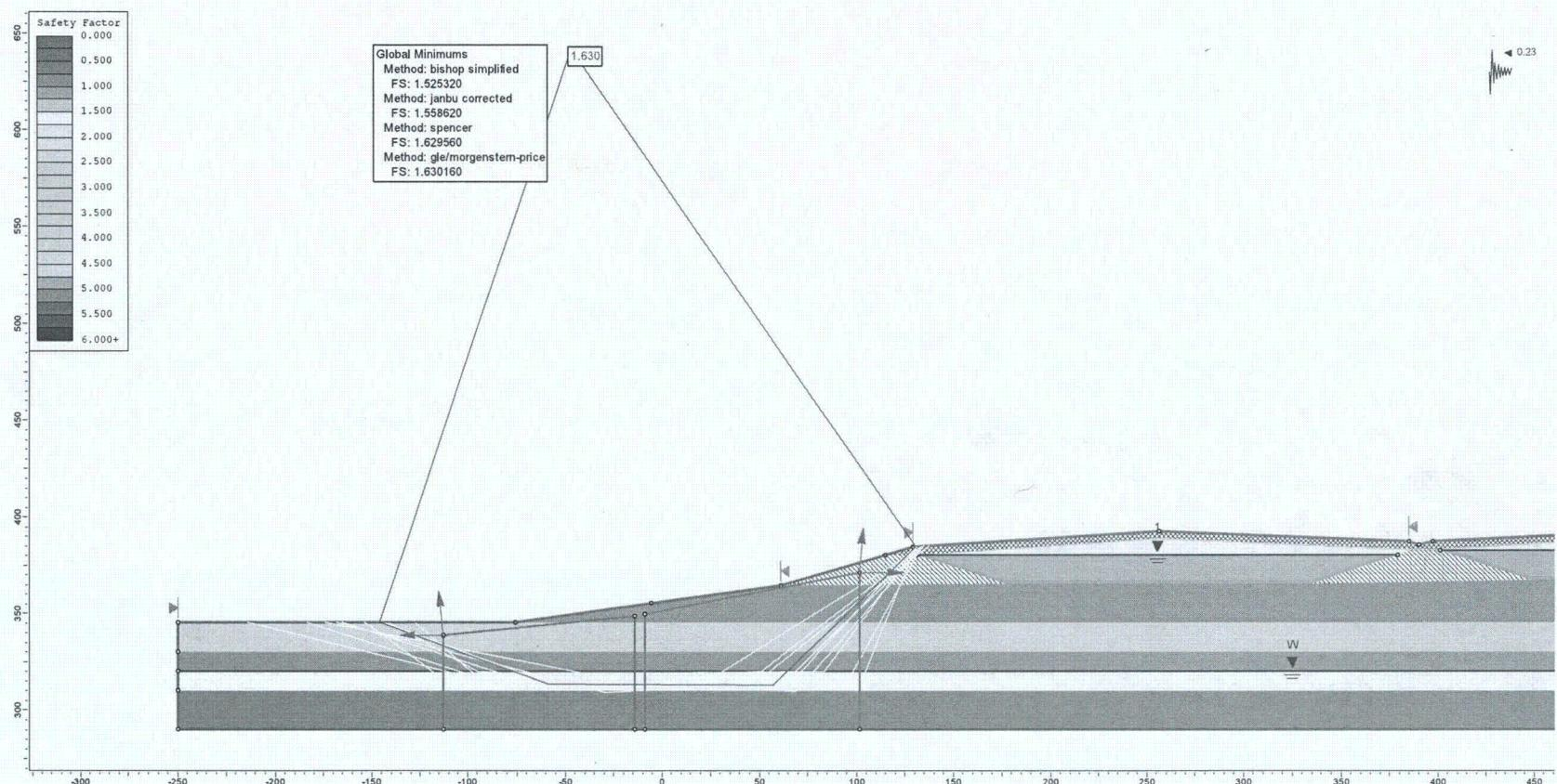
**Figure F4.** Pseudo static analysis of the exterior berm in a 475-year event assuming partly liquefied state in the lower sand (wedge failure surface,  $k_h = 0.67 \times \text{PGA}$ ).
