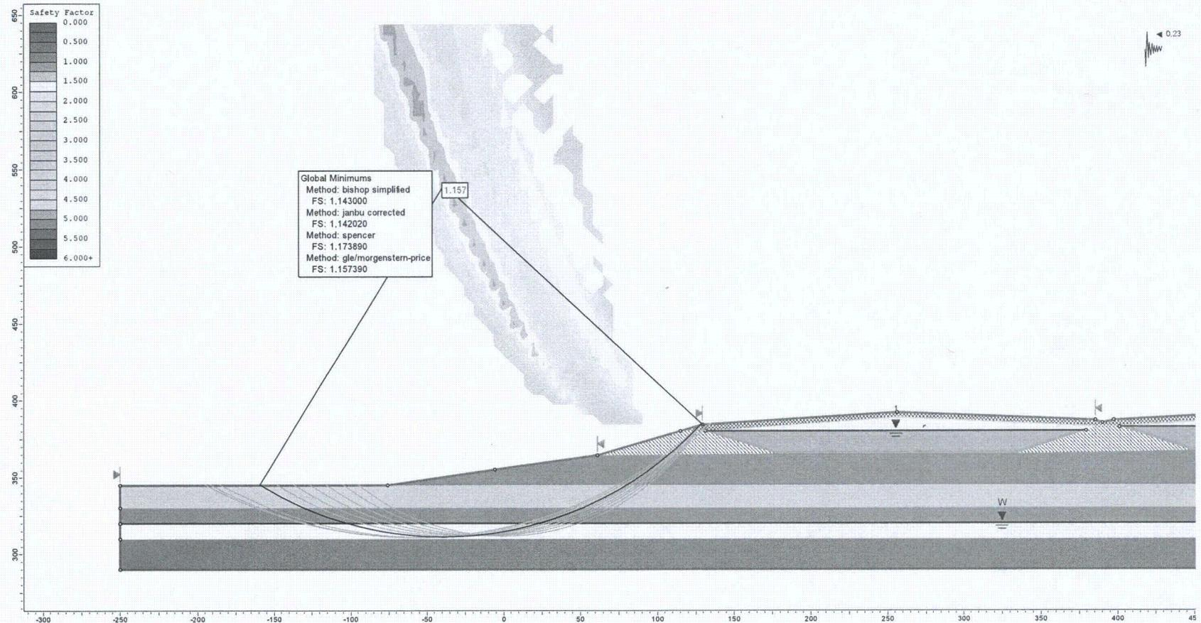
**Figure F1.** Pseudo static analysis of the exterior berm in a 475-year event assuming full liquefaction in the lower sand (circular failure surface,  $k_h = 0.67 * \text{PGA}$ ).
