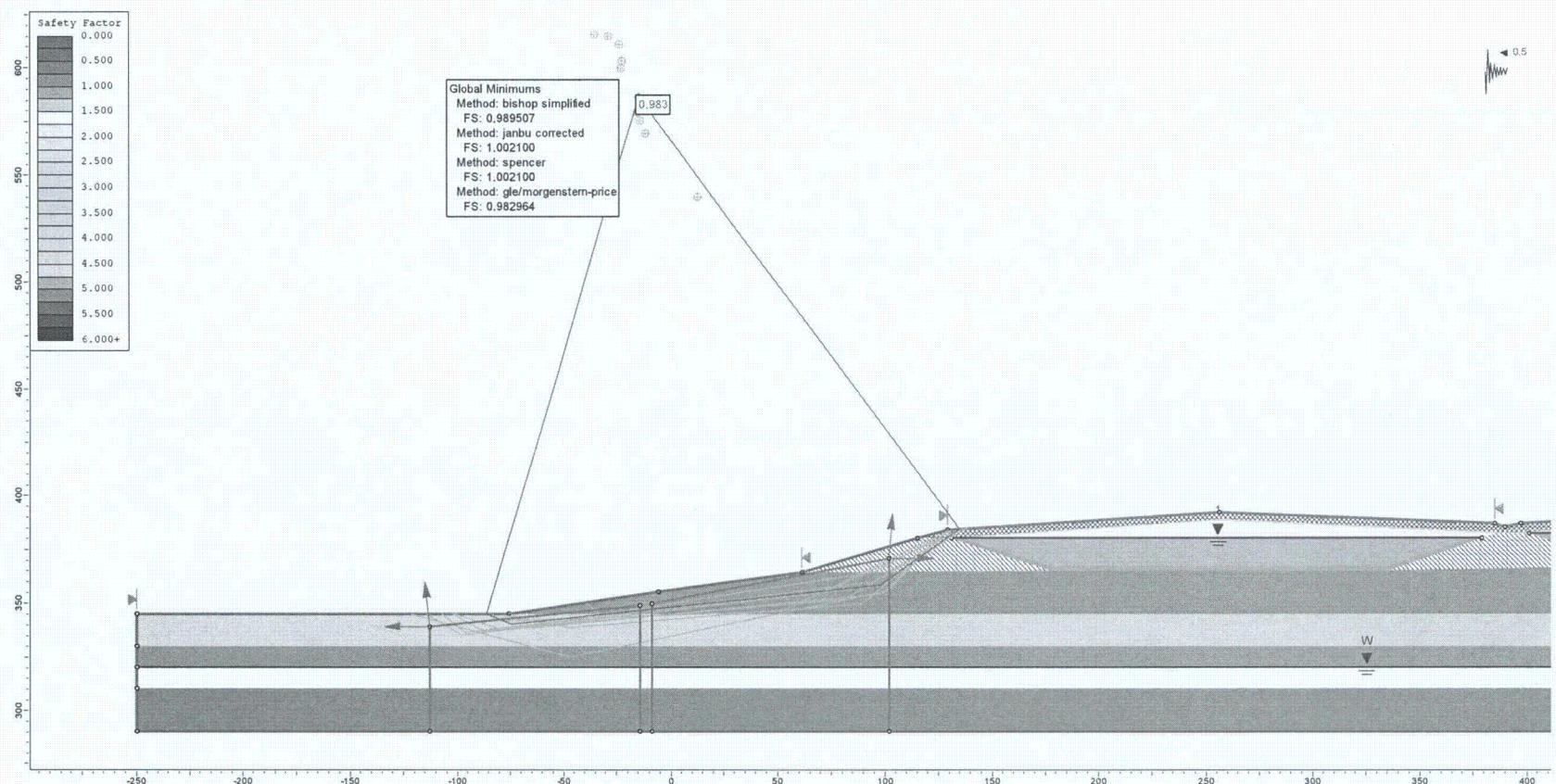
**Figure F24.** Pseudo static analysis of the exterior berm in a 2475-year event assuming no liquefaction in the lower sand (wedge failure surface,  $k_h = 0.5 * \text{PGA}$ ).
