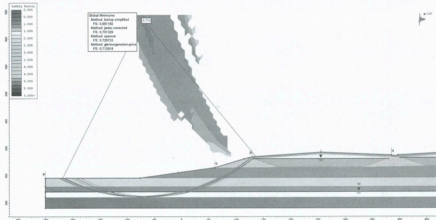
**Figure F15.** Pseudo static analysis of the exterior berm in a 2475-year event assuming partly liquefied state in the lower sand (circular failure surface,  $k_h = 0.67 \times \text{PGA}$ ).
