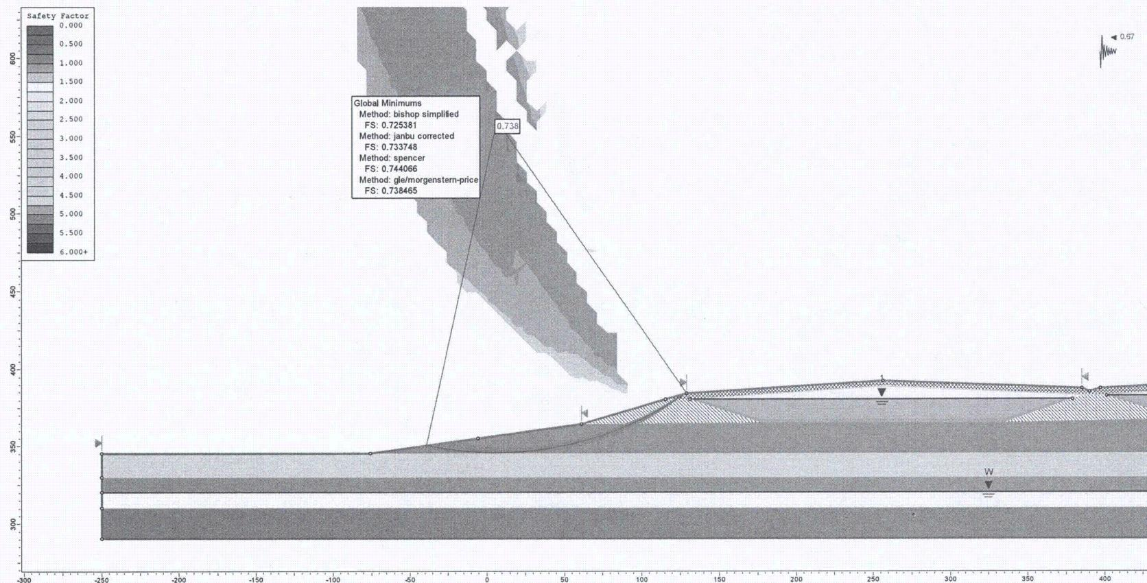
**Figure F17.** Pseudo static analysis of the exterior berm in a 2475-year event assuming no liquefaction in the lower sand (circular failure surface,  $k_h = 0.67 * \text{PGA}$ ).
