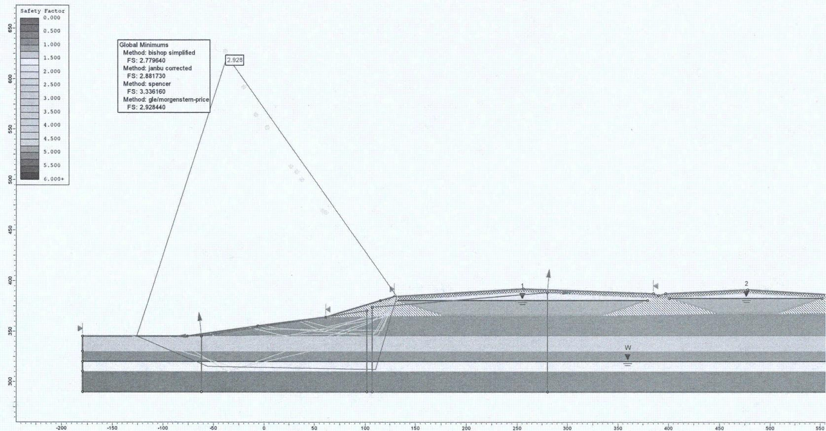
**Figure E3.** Post-liquefaction stability of the exterior berm assuming the lower sand layer in fully-liquefied state (wedge failure surface).
