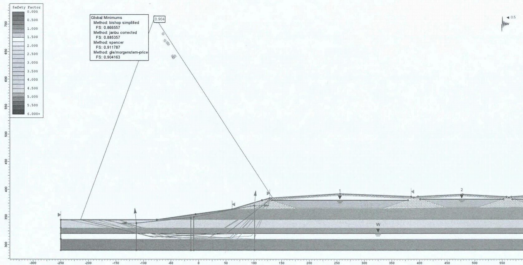
**Figure F22.** Pseudo static analysis of the exterior berm in a 2475-year event assuming partly liquefied state in the lower sand (wedge failure surface,  $k_h = 0.5 \times \text{PGA}$ ).
