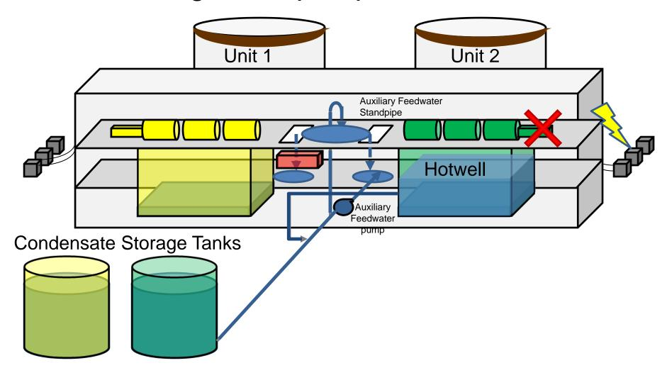
Circulating water pump circuits in the cabinet were damaged and caused 2 of the 3 Unit 1 circulating water pumps to trip off
