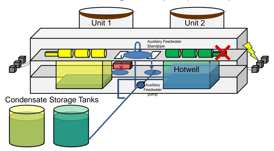
The loss of 2 circulating water pumps resulted in a loss of condenser vacuum, which caused the Unit 1 reactor to trip
