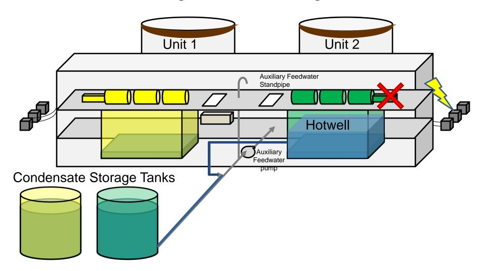
Auxiliary Feedwater pumps began injecting into the Steam Generators following the Unit 2 reactor trip, as designed
