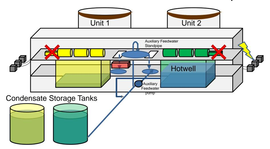
The condenser could not be used for decay heat removal, so main steam relief valves were used, as designed
