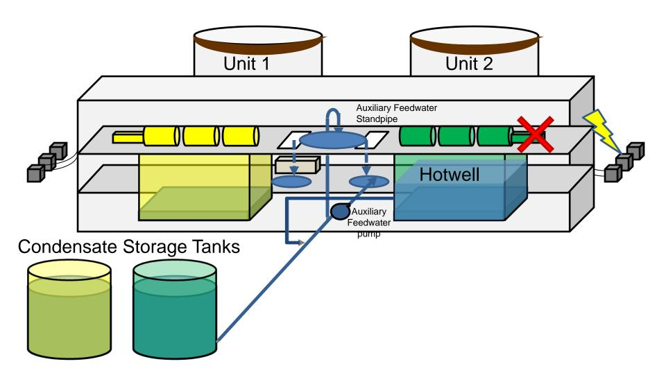
The water entered a non safety-related electrical cabinet that contained Unit 1 circulating water pump electrical circuits
