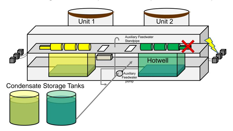
The Unit 2 Turbine Trip caused water in the hotwell to reject to a pipe leading to the Unit 2 Condensate Storage Tank, as designed
