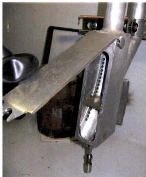
Figure 10.6 Pneumatic Transfer System Terminus
