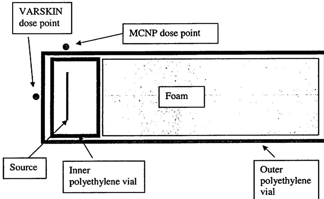
Figure 1. Schematic of source configuration.
