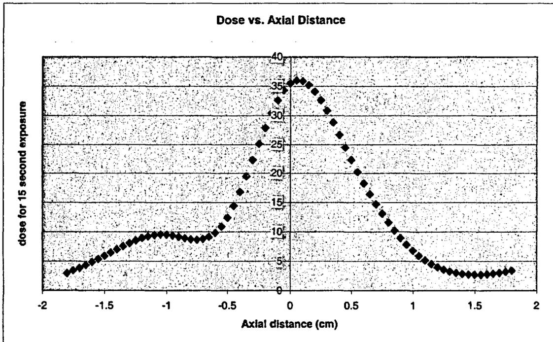
Figure 5. Spline fit of dose versus axial position along vial
